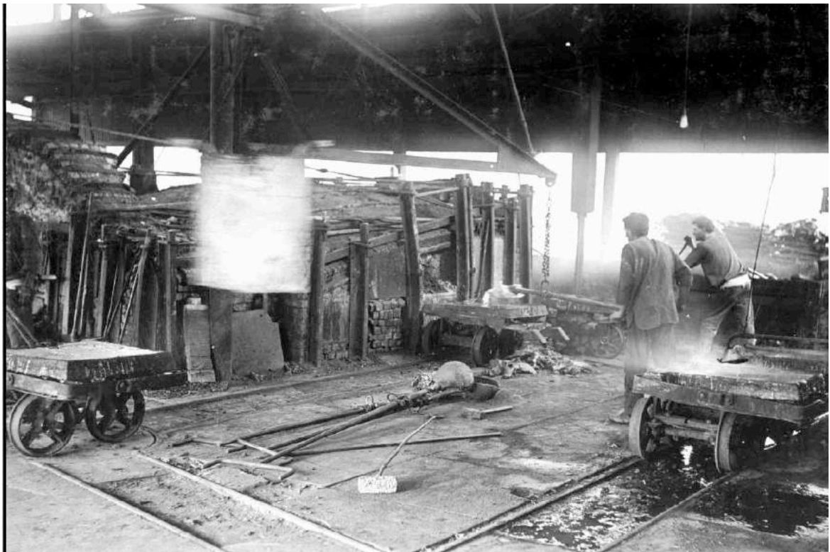
Fig 15 Casting copper anodes for the electrolytic refinery (PIRSA N020506a)
