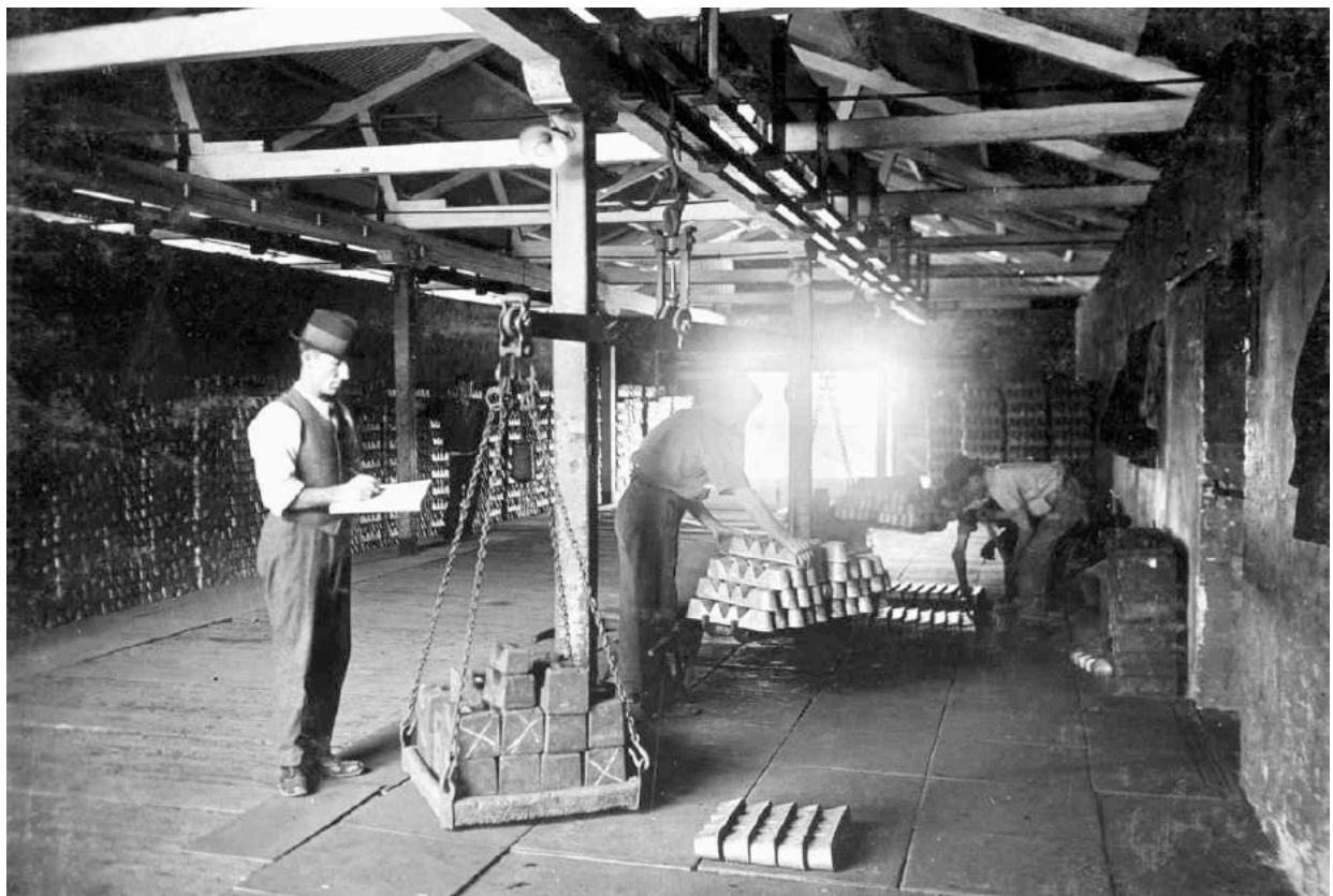
Fig 9 Weighing finished ingots in the copper store (PIRSA N020500a)
