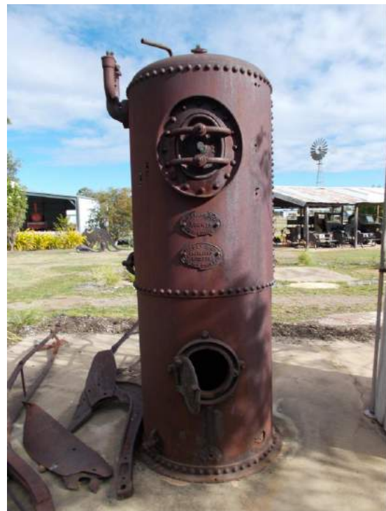
Vertical boiler 'Robey and Co. Engineers No. 12772 Lincoln England', also badged: 'Smellie and Co, agents,
