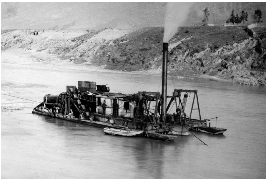
Figure 1: The Dunedin, the first fully engineered steam dredge in New Zealand.
