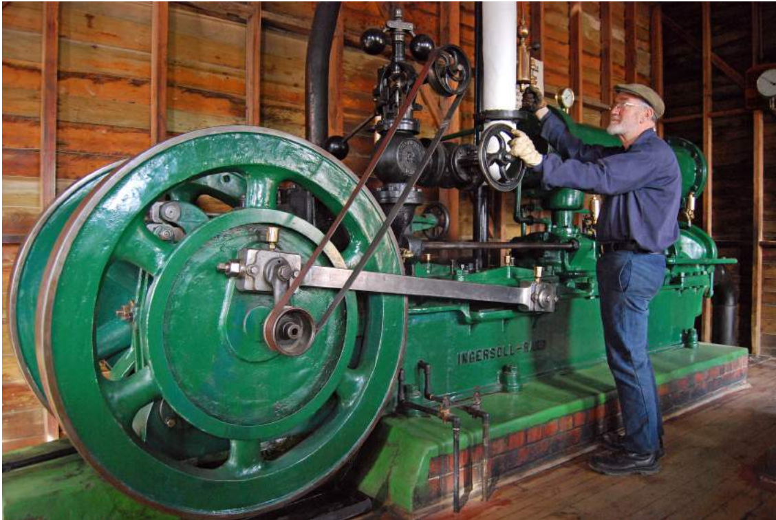
Figure 7: The Ingersoll-Rand tandem two-stage air-compressor.
