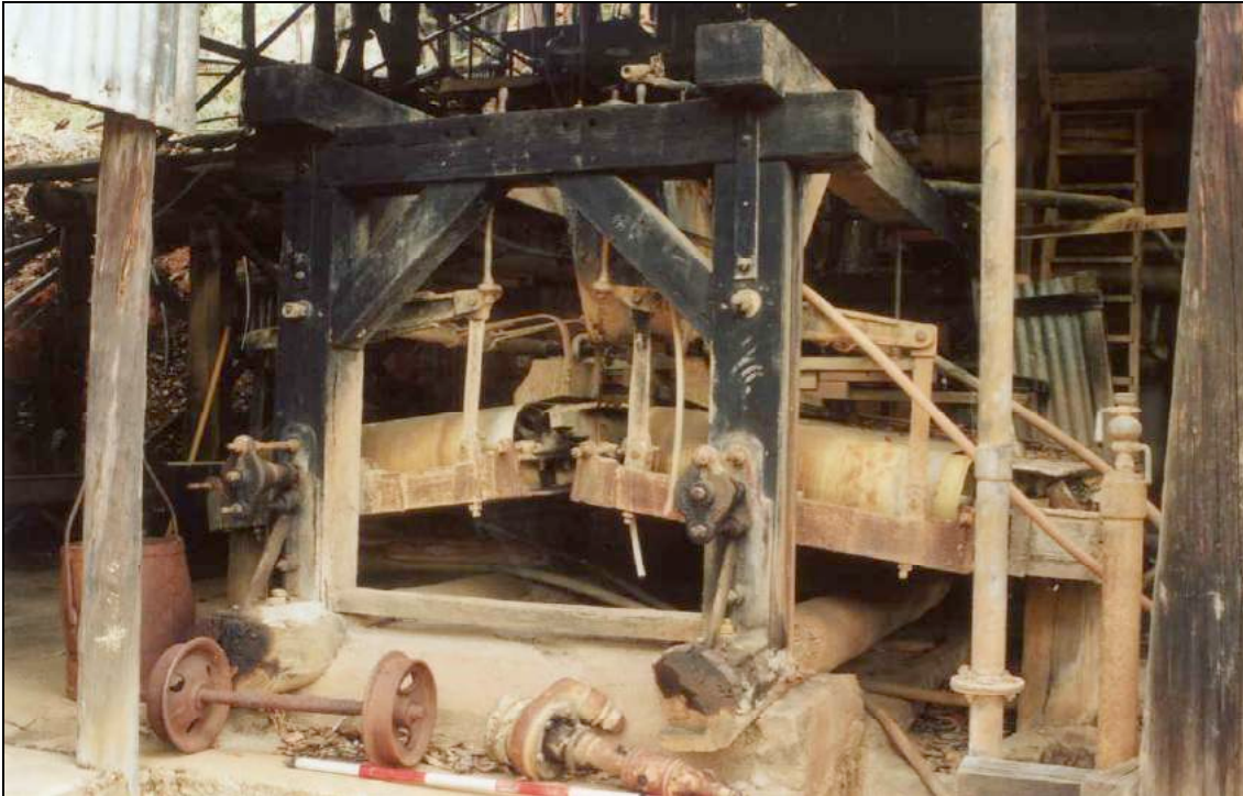
Figure 4: Luhrig Vanner, Emuford mill
