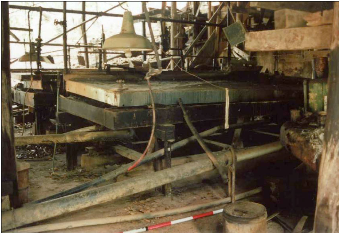
Figure 5: Krupp Shaking tables, Emuford mill
