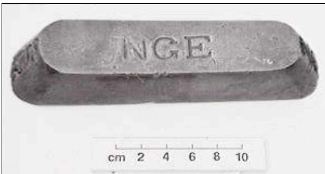
Figure 6: Ingot of Nymagee copper with the brand NGE ca. 1884.
