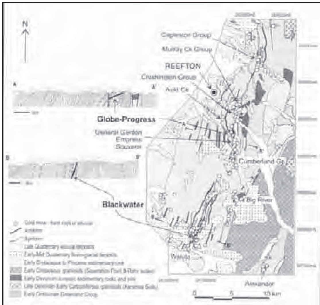
Geological map of the Reefton area showing the locations of the gold-quartz vein and alluvial gold mines (after Cox et al., 2002). Cross-sections through the Globe-Progress (A-A') and Blackwater (B-B') deposits. After Christie et. al. 2006).
