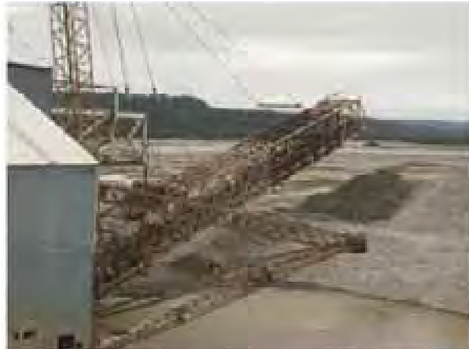
FIG 6 - Stacker depositing the tailings (photo courtesy of Birchfield Minerals/Stewart Nimmo Photography).
