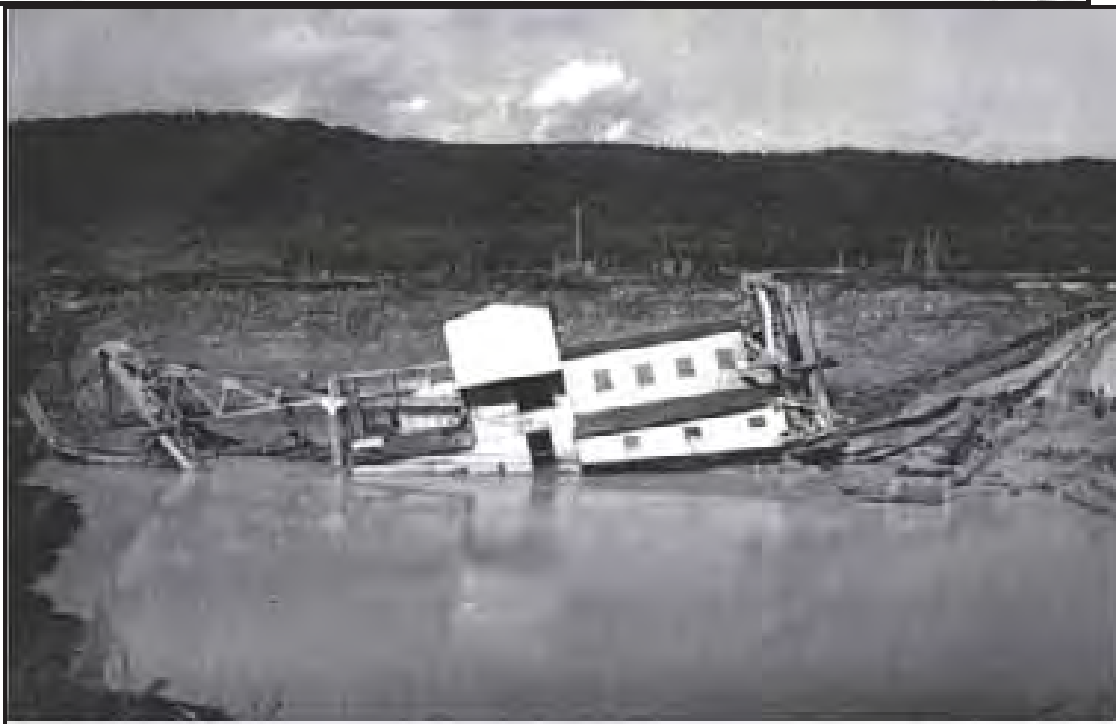
A crewman was drowned when the Arahura dredge sank in its pond on 5th of March 1949. The incident is attributed to the collapse of the digging face on to the bow of the dredge. It was dismantled and rebuilt. Digging recommenced in January 1953.
