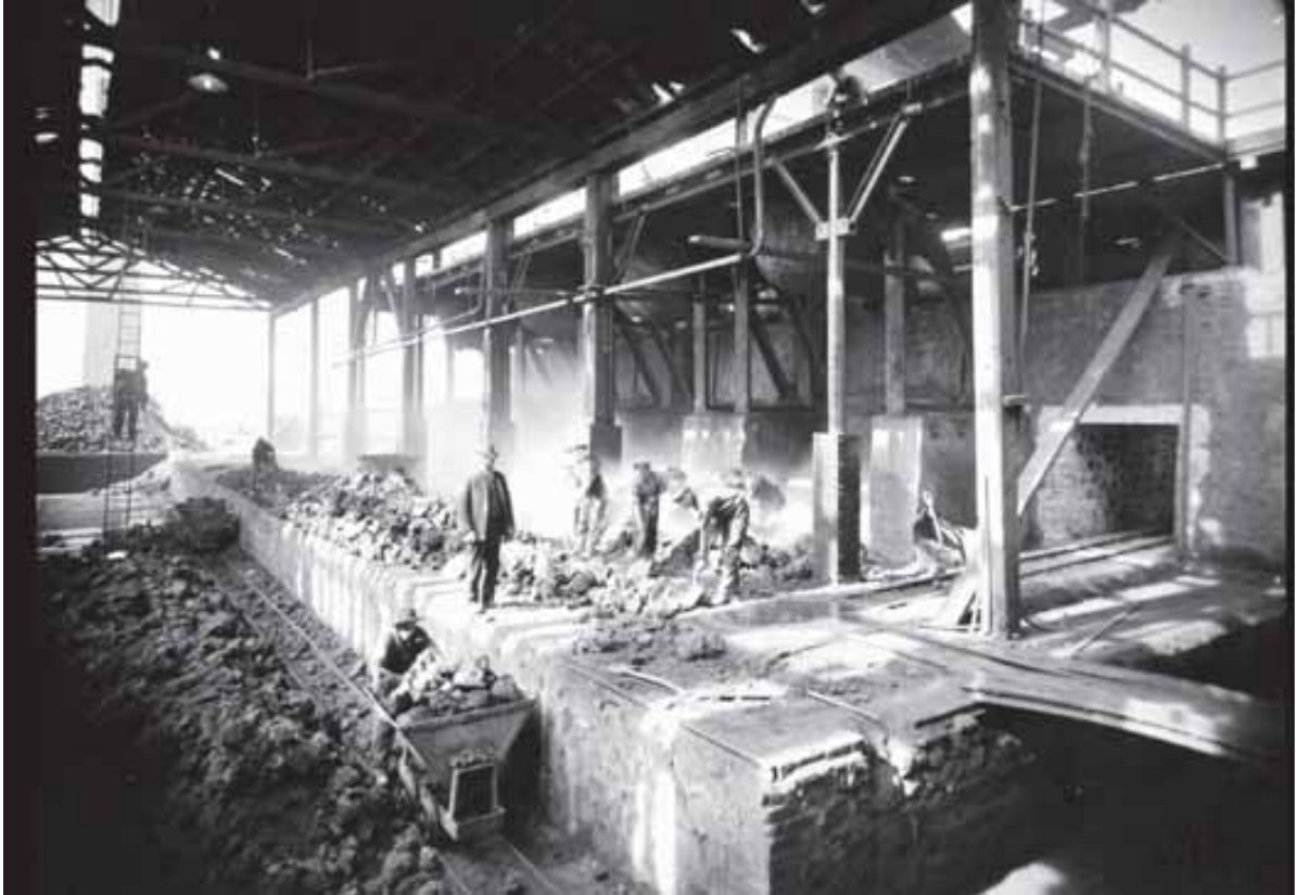
Fig 11 Breaking up sintered ore for the blast furnaces (PIRSA 044487a)
