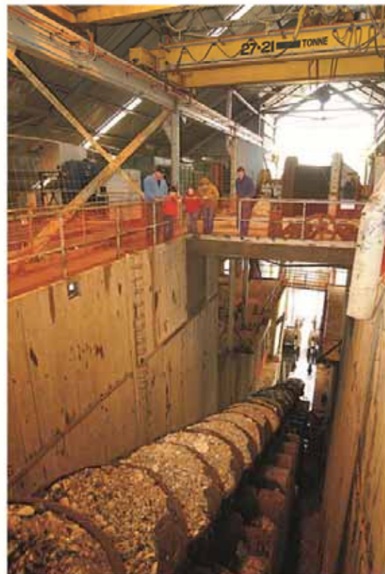
FIG 4 - Bucket line with 0.57 m 3 buckets (photo courtesy of Birchfield Minerals/Stewart Nimmo Photography).
