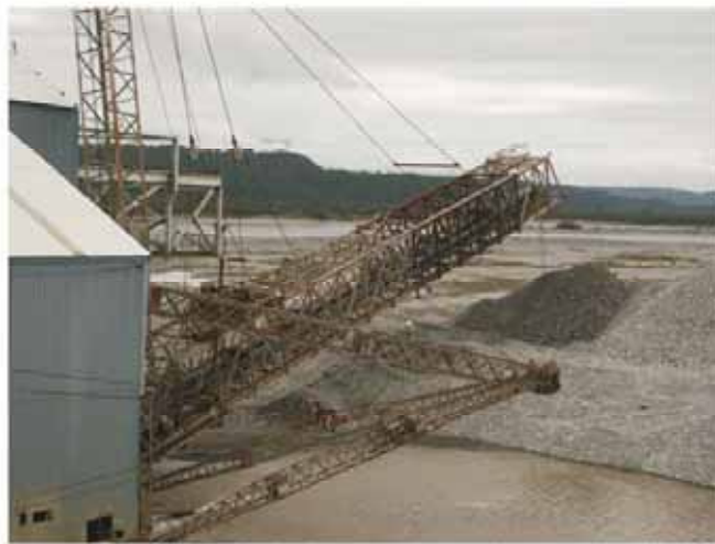
FIG 6 - Stacker depositing fine tailings (photo courtesy of Birchfield Minerals/Stewart Nimmo Photography).
