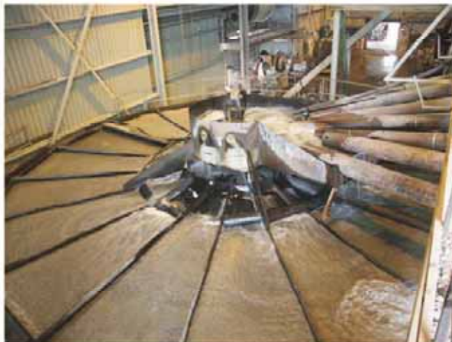
FIG 7 - Radial jig in operation (photo courtesy of Birchfield Minerals/Stewart Nimmo Photography).
