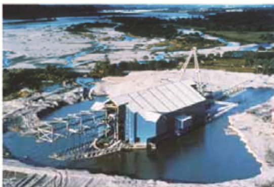
FIG 1 - The Grey River dredge operated by Birchfield Minerals Ltd at Ngahere. The dredge is 150 m long from the front A frame to the end of the stacker and reaches 30 m above the water line.
